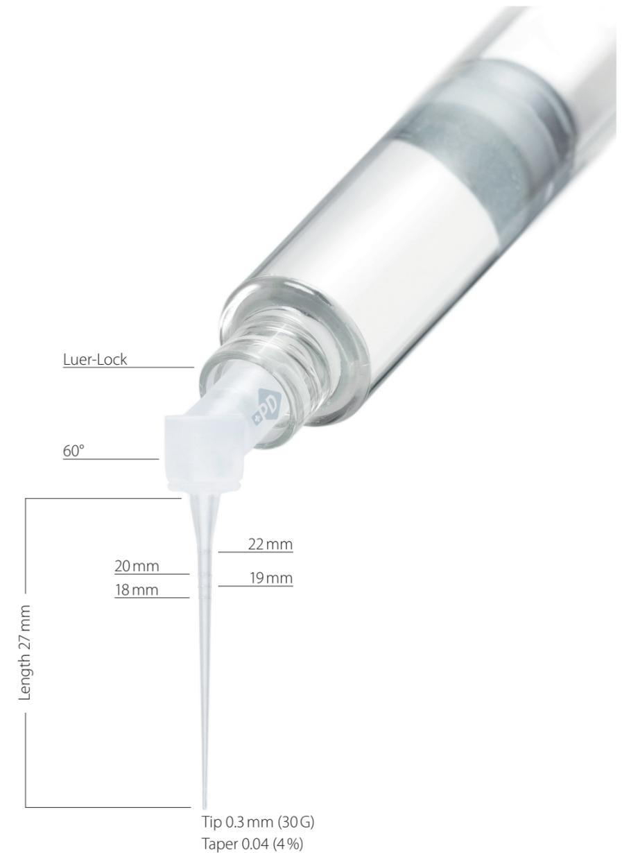
*IrriFlex® offers the benefit of being able to be inserted very deeply into the most curved root canals without the risk of extrusion into the periapex. Mounted on a 5 ml Luer-Lock syringe, the orientation of the lateral openings located on the same plane 0.5 mm from its end creates useful shear stress forces to eliminate the smear layer and disorganize bacterial biofilms from the root canal walls.*
